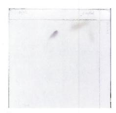
Loaded 25  $\mu g$  TDM and developed 1st dimension 100/14/0.8 chloroform/ methanol/ water, left to right.
