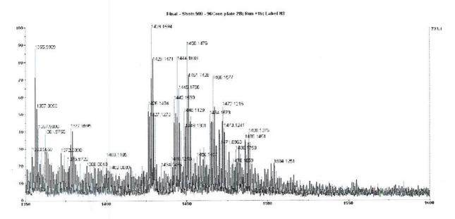
Purified sample (1  $\mu$ l at 1  $\mu$ g/ $\mu$ l) was mixed 1:1 with DHB matrix and analyzed in positive electrospray mode.
