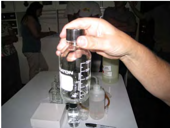
Figure 5.1.3.3: Coating the bottom of the bottle
