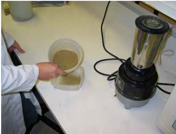
Figure 10.1.1. Preparing food. Use a general laboratory grinder (pictured here), a grinding mill or a household coffee grinder. To ensure food is small enough for the earliest stages, use a sieve with holes no larger than 250 microns in size.
