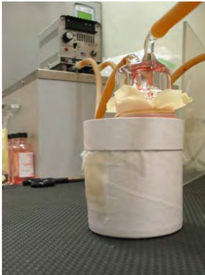
Figure 2.4.10.2. Example of a membrane feeder using dental dam and an electric pump and heater to circulate warm water.
