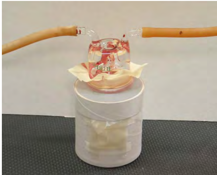
Figure 2.4.10.2. Example of a membrane feeder using dental dam and an electric pump and heater to circulate warm water.
