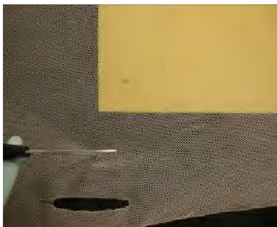
Figure 5.1.4.2.2: Cutting the sample ensuring that there is a generous amount of material left around the template.
